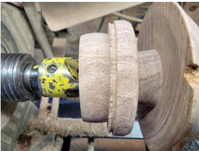
#6 Tenon is Beveled on Both Ends to Swivel in Chuck Jaws
