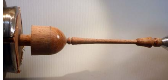
Figure 29. Waste is parted off
