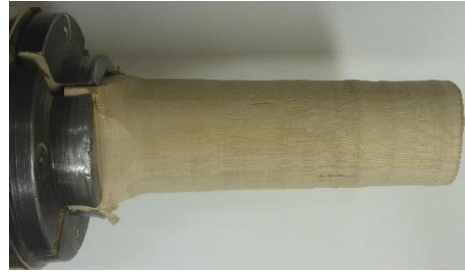
Figure 2. Billet rounded, check for defects
