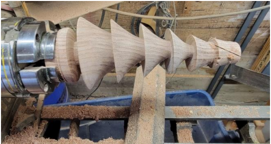
#12 Set Up on Point 1 Saw the tip off with the turned angle
