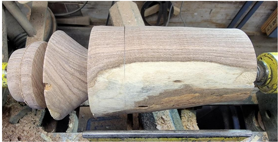
#5 Turning section 1 (Tenon, Tree Base and Lower Tree Branch's)
