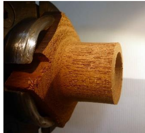
Figure 33. Jam chuck recess cut
