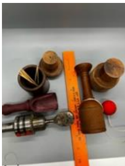
Jacob chuck with modified spade bit Scoop, toothpick holder with jam chuck Bilboquet and jam chuck
