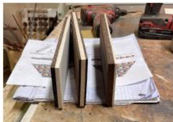
d. After glue is dried, clean up boards.
