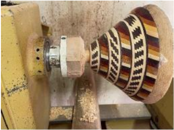
g. Cut bowl 2 off lathe.
