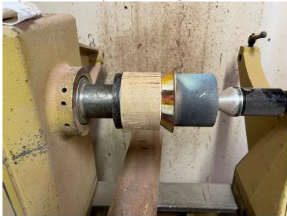
a. Glue base to waste block
