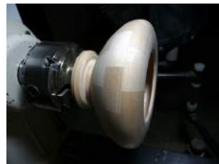
Finish-turn the outside and inside
